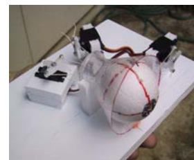
Figure 16. An eye equipped with a camera and a log-polar sensor, which is actuated by three motors. The whole device obeys Listing's law (von Helmholtz, 1955).
